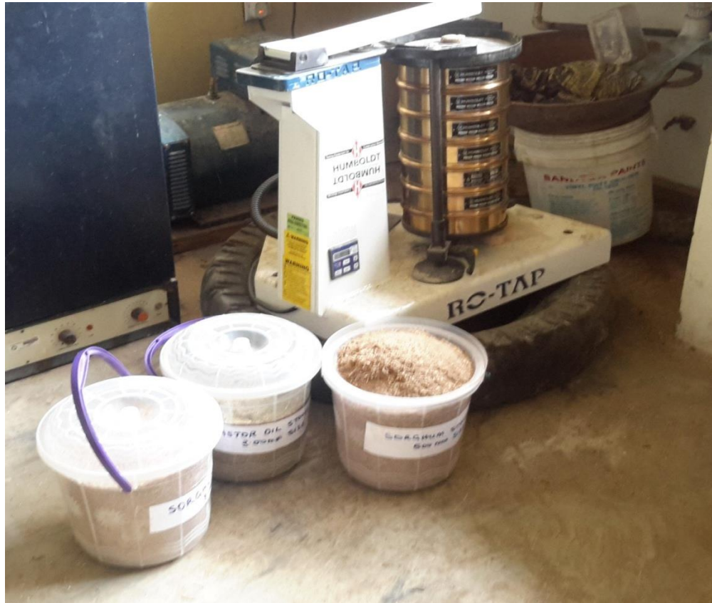
Figure 8: The sieve shaker Apparatus and the sample for the determination of particle Size distribution
